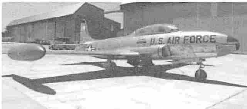
The T-33 with its wing tanks in place.
